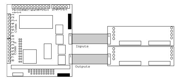
The diagram above shows the location of pin 1 on the ribbon cables that connect to the relay cards.
