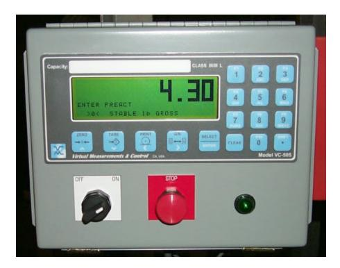
Next enter the preact value and press the **ENTER** key. The preact value is sometimes referred to as the "product in stream at cutoff" or "after flow". The preact has the effect of closing the catch gate early. For a bag weight of 50.00 lbs. & a preact value of 4.30 lbs., the catch gate will close when there is 45.70 lbs. in the bag (50.00 - 4.30 = 45.70).
