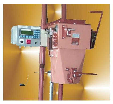
Model DMC-17 load cell conversion kit will convert Howe Richardson Model G-17 & Express Scale Model GB-25/32 mechanical beam bagging scales into a digital load cell scale.
