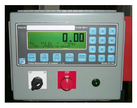
The load cell controller has (15) memory locations to store different bag weight settings. To enter the weight data into memory, begin by pressing the **F1** key.
