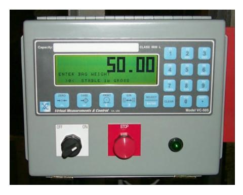
Enter the target bag weight and press the **ENTER** key.
