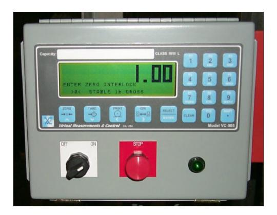
Enter the **Zero Interlock** value and press the **ENTER** key.
